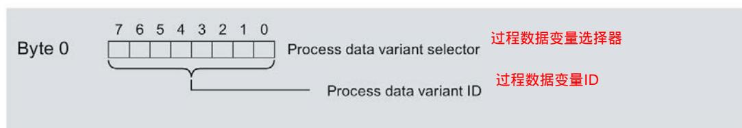
Figure C-4 Assignment of the control byte for Process data variant selector (Byte 0)
