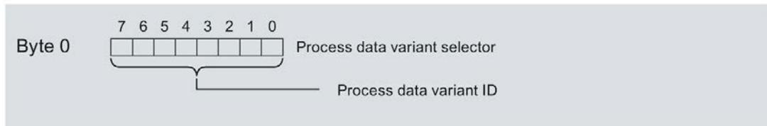
Figure C-8 Assignment of the control byte for Process data variant selector (Byte 0)
